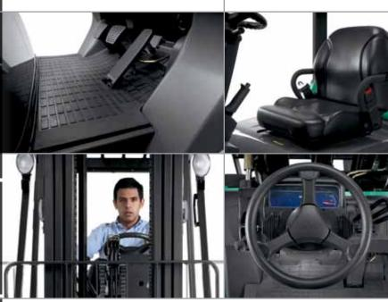
The FG15N-FG35N / FD20N-FD35N series is built to help protect the operator and surrounding personnel. Each unit comes standard with the Integrated Presence System (IPS), which is designed to disengage all powered travel and some hydraulic functionality when the operator leaves the normal operating position. Additionally, warning alarms sound and indicators are shown on the display panel, informing the operator and surrounding personnel that the system is engaged.
