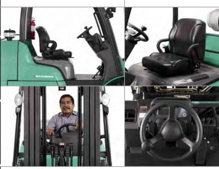
The FG40N1-FG55N1 / FD40N1-FD55N1 series is built to help protect the operator and surrounding personnel. Each unit comes standard with the Integrated Presence System (IPS), which is designed to disengage all powered travel and some hydraulic functionality when the operator leaves the normal operating position. Additionally, warning alarms sound and indicators are shown on the display panel, informing the operator and surrounding personnel that the system is engaged.
